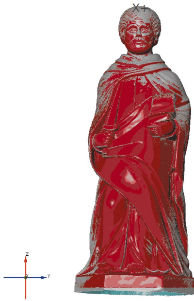
Figure 12. Overlay of the original statue (in red) and the BIS replica (in grey)
