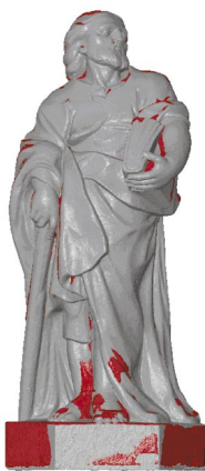
Figure 7. The results indicate surface deviation of the stone replica from the original statue as a colour map
