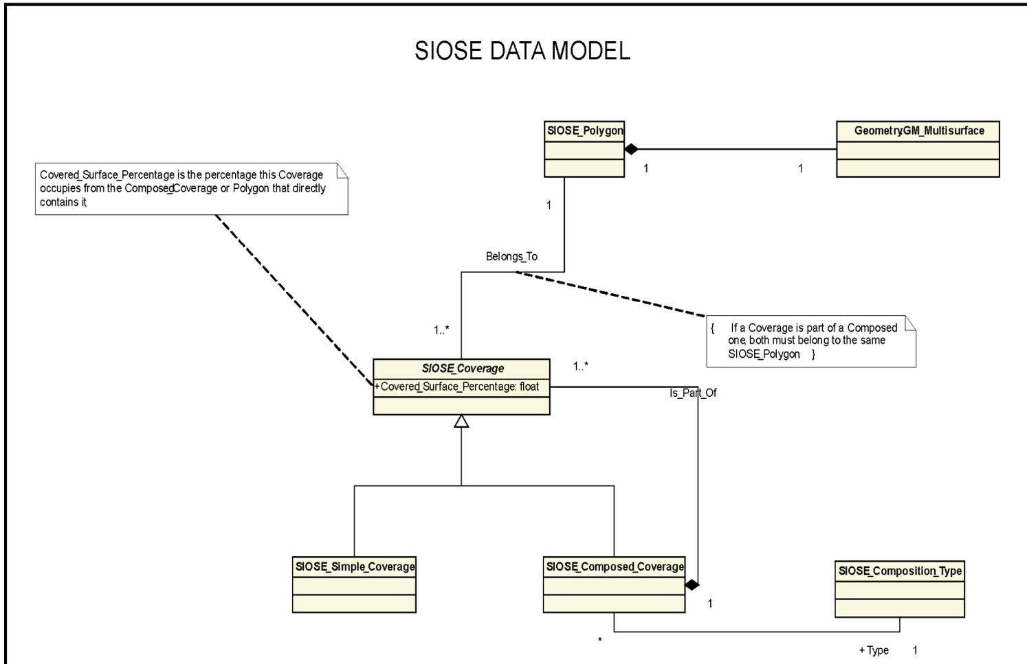
Fig. 5. SIOSE core data model
