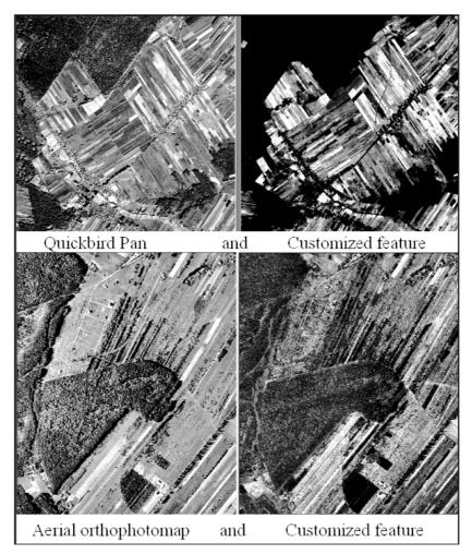
Fig. 3. Two top images; a QuickBird PAN band and the visualization of the customized feature (from Fig. 1). Below the same customized feature on a subset of the 8-bit orthophotomap from a scaned aerial imagery (B&W, scale 1:13.000)
