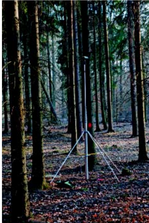
Figure 2. Aluminum pole with GNSS receiver
