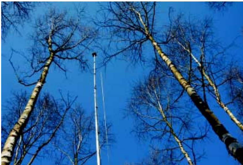
Figure 3. GNSS receiver gather data on 15 meters height
