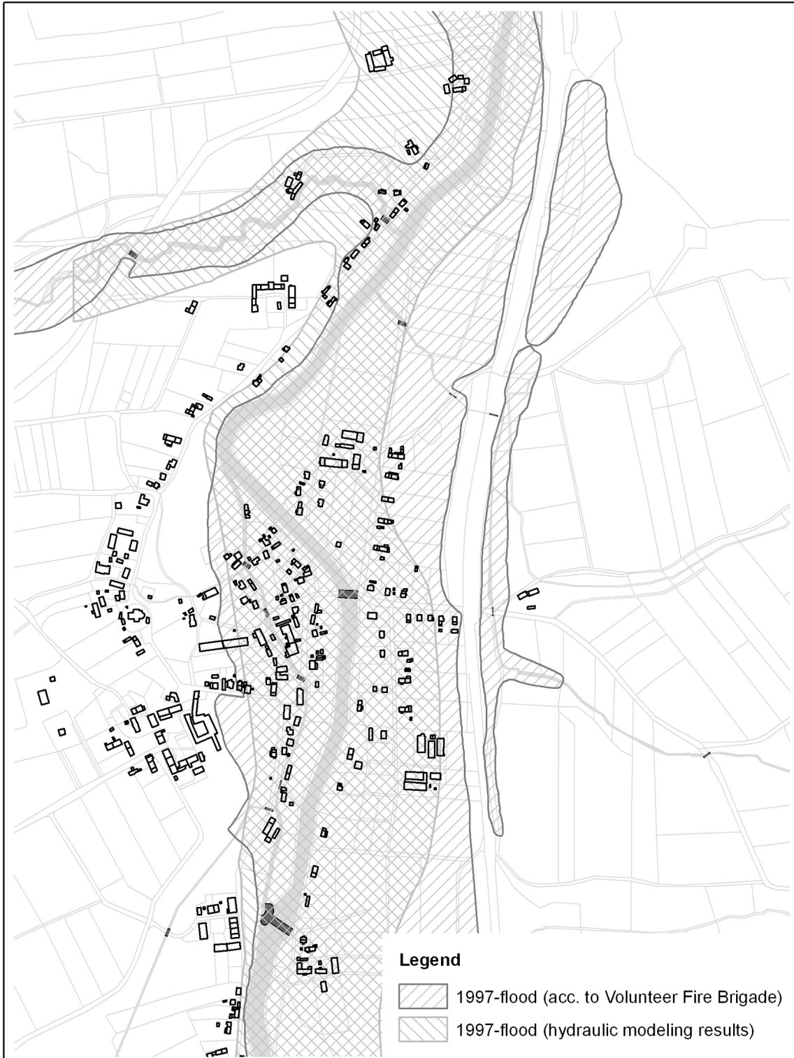
Figure 1. Gorzanów center – Comparison of inundation extents from field surveys and hydraulic modelling, for 1997 flood
